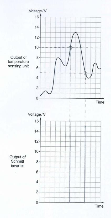
Use the axes provided to draw the corresponding output signal of the Schmitt inverter, when the signal from the temperature sensing unit is applied to its input. [3]
