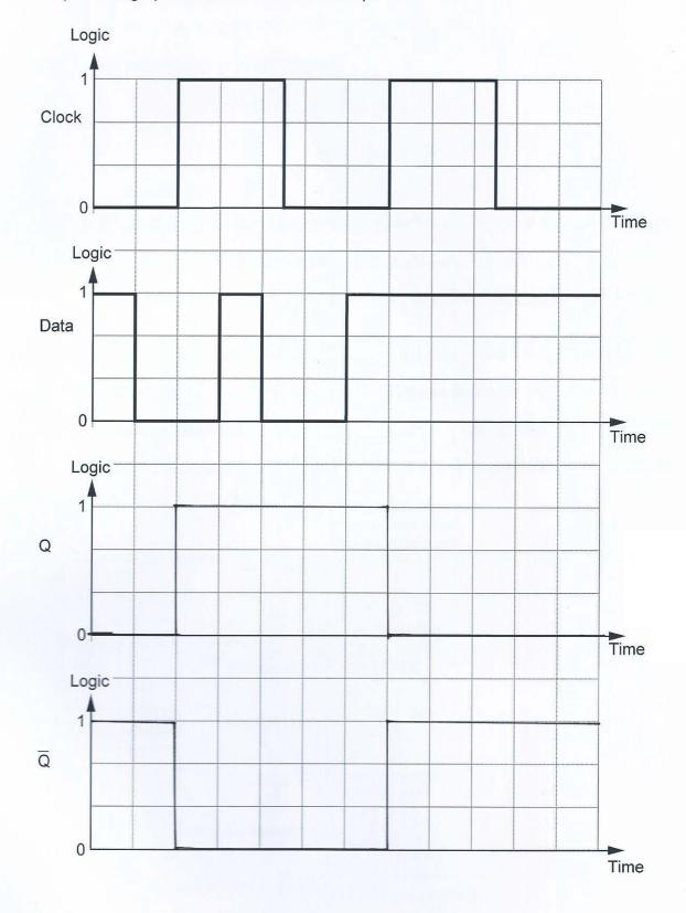
**10.** A rising-edge triggered D-type flip-flop is used for data transfer.
